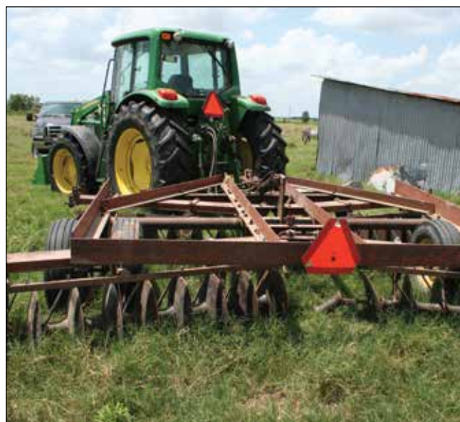
Figure 14. Disking implements can be used to break up the top 2-4 inches of soil. (Photo courtesy of Blake Alldredge, Texas A&M AgriLife Extension Service)
